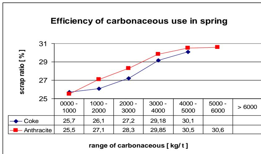
Fig. 3 Efficiency of carbonaceous use in spring time
