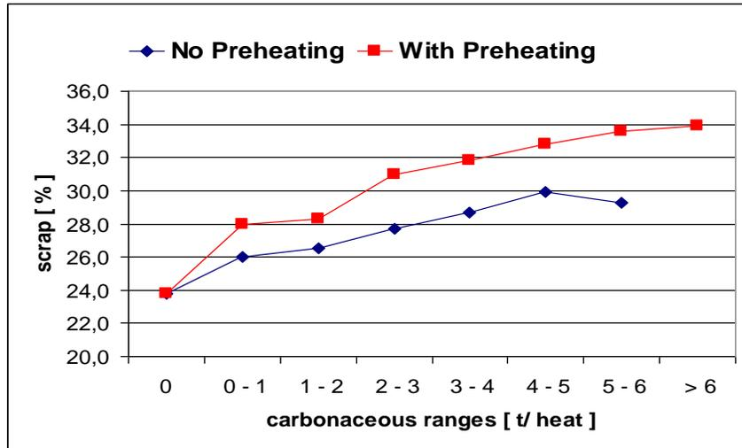
Fig. 4 Efficiency of carbonaceous use at scrap preheating
